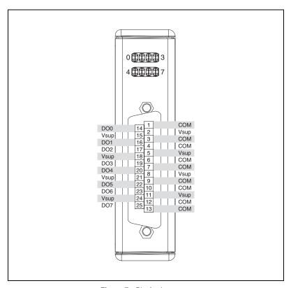
Figure 7. Pin Assignments
